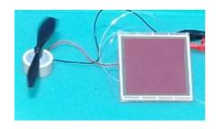
Dimensions: Length: 1...15 cm Width: 1...15 cm Thickness: 0.5...4.5 mm Voc: 0.5 V Maximum power density: 7 µW/cm<sup>2</sup> @ 200 lx
